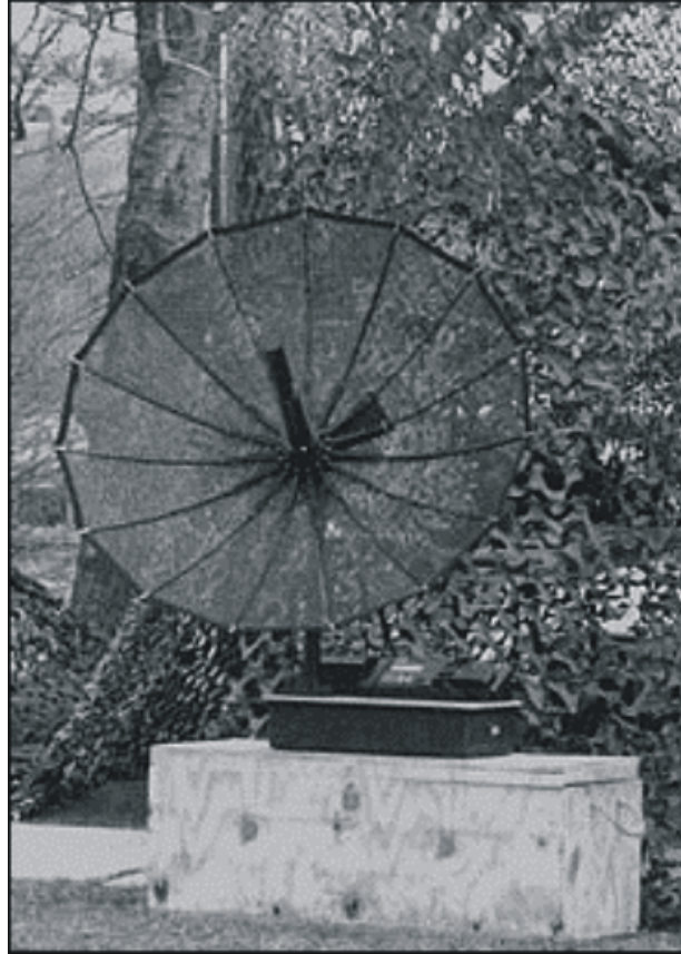
Figure C-4. Satellite Telecommunications System
