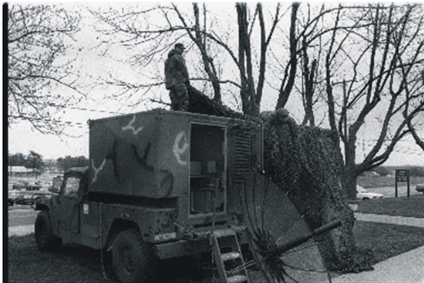
Figure C-3. Climate-Controlled S-250 Shelter
